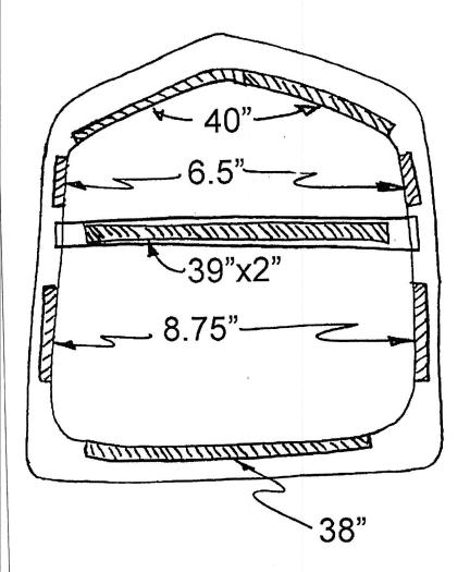
Note: All pieces are stapled except the 39"X2" piece which is glued. Since the hood skin is already on the frame, you must put new staples in by hand and bend over with pliers. Alternatively, you can leave the old staples in, and simply glue all the pads in.
